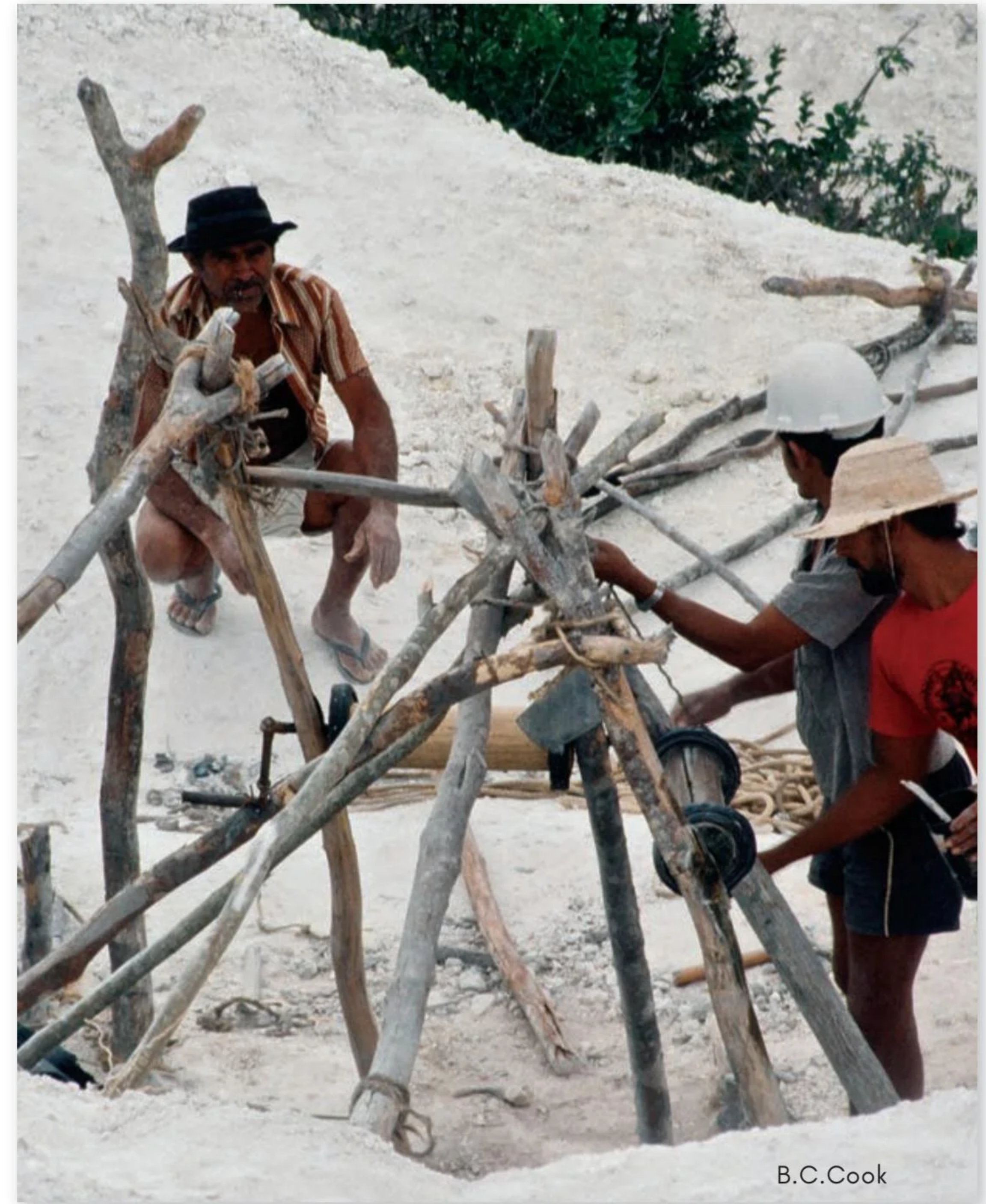
This is the assembly to haul the excavated vein material to the surface. Thousands of tons of material were brought out bucket by bucket. Over the years, the miners created several kilometers of steep shafts and interconnected drifts by hand. The only way down was by holding a rope and rappelling at a steep angle.
