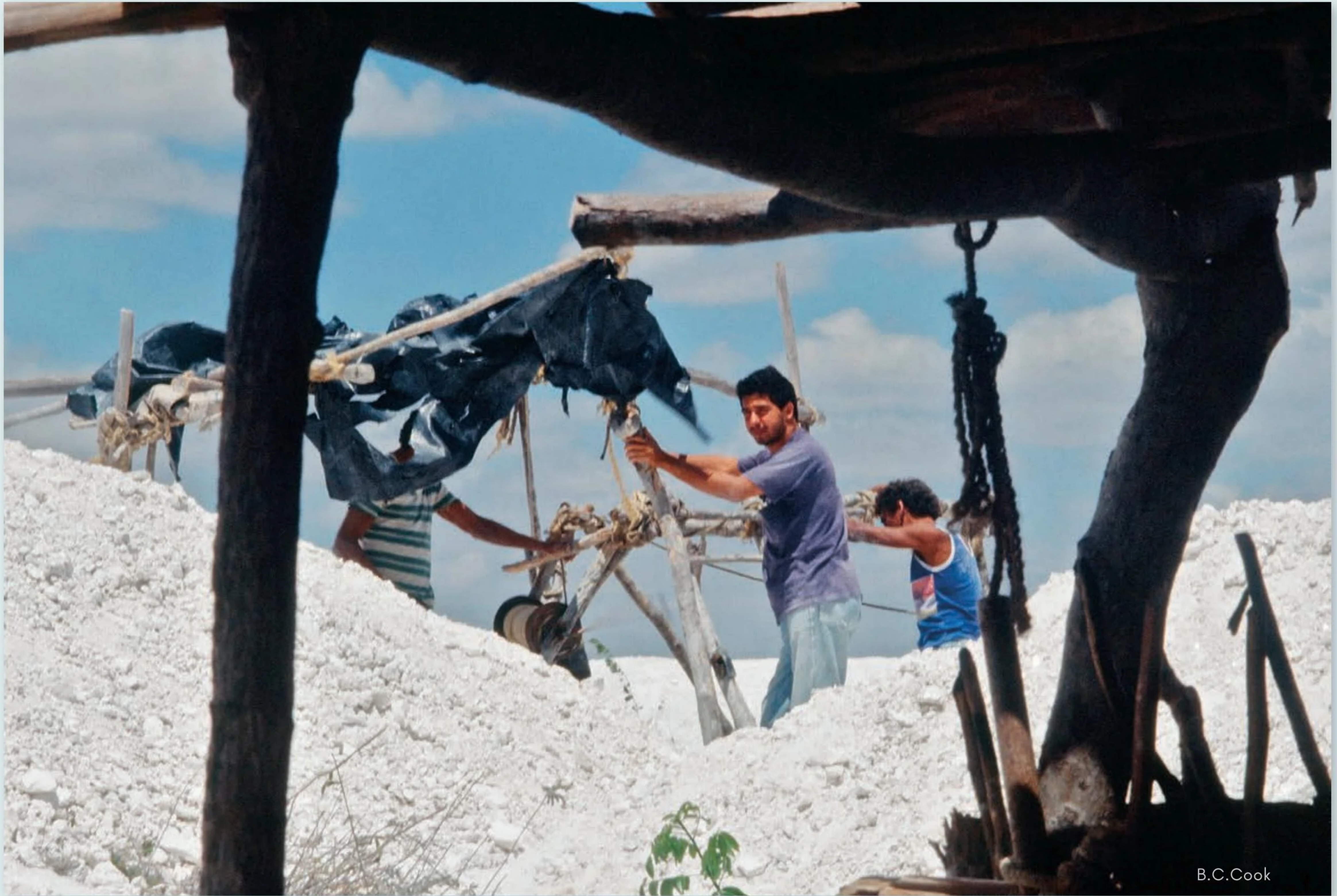
Using basic tools such as sticks, rope and bits of tire rubber, these men built the Batalha Mine's infrastructure.
